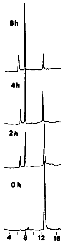
Fig. 1. Reverse-phase HPLC profile showing furin catalysed cleavage of proalbumin peptide A (normal). 1 nmol samples of peptide were analyzed after 0, 2, 4 and 8 h incubation with furin (0.25 fM); 3 \mu C-18 column, detection at 215 nm; other details in text.
